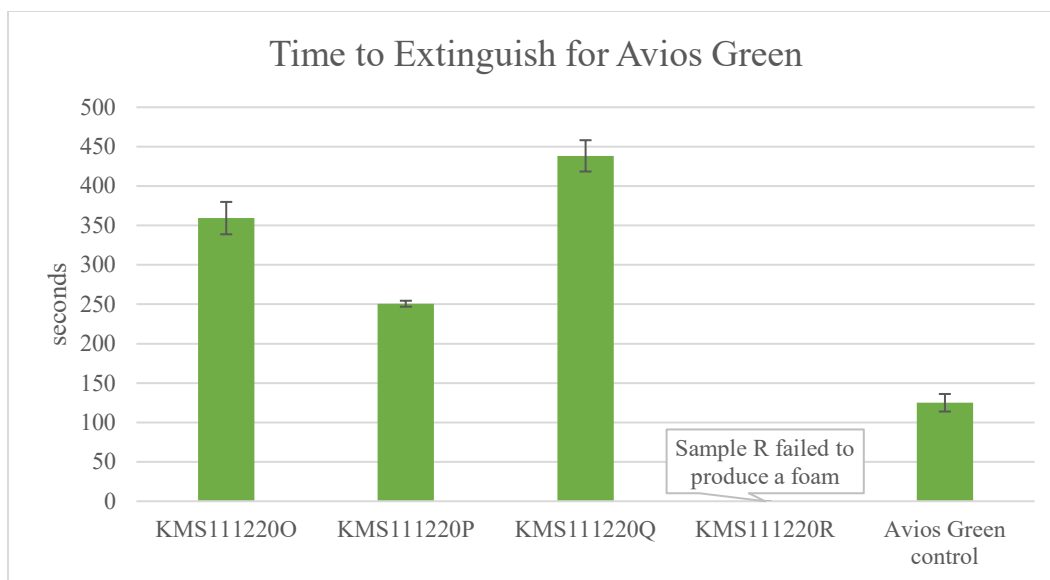
Figure 17. Total extinguishment time for Avios Green with formulations from table 2.
