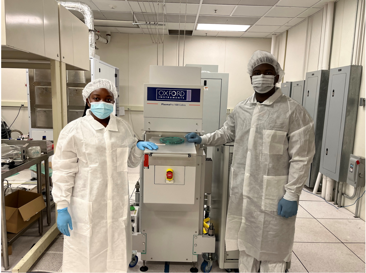
Figure 1. The PlasmaPro 100 Cobra ICP etching system installed in the clean room in the Engineering building at the Alabama A&M University.
