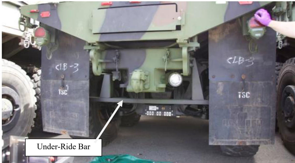
Figure 11. MTVR Under-Ride Bar Location at Rear of Vehicle Provides Unused Mounting Holes for Test Fasteners and Ready Access to Corrosive Environment
