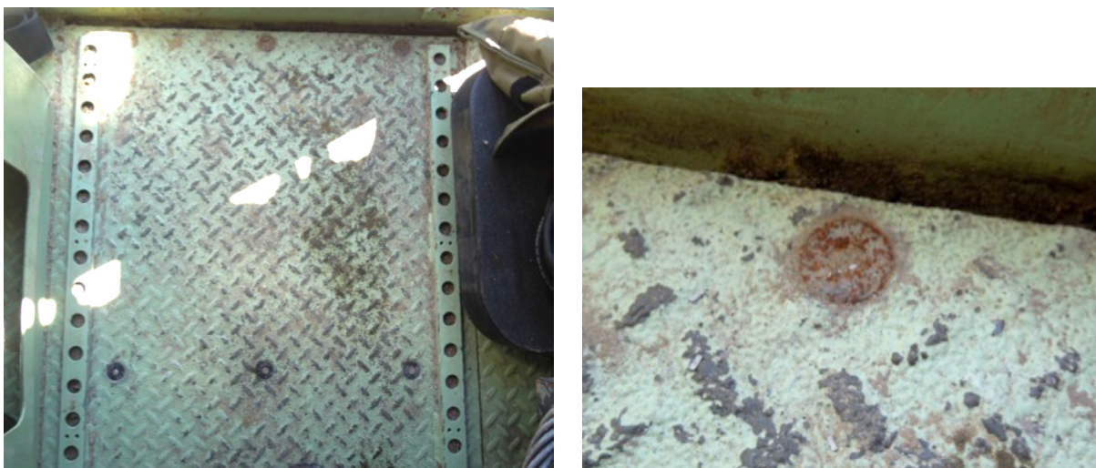
Figure 8. MRAP Access Panel Screws Illustrating in Field Corrosion Issues
