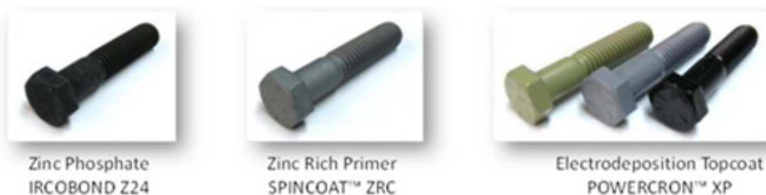
Figure 1. Coating Layers of Zinc Rich/Electrocoat System Consisting of Zinc Phosphate Pretreatment (Left), Inorganic Zinc Rich Primer (Center) and Electrocoat Topcoat (Right)
