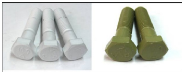
Figure 3. High Purity Aluminum Plating on Steel Fasteners (Left), and Similar Fasteners with the Addition of an Electrodeposition Topcoat (Right)
