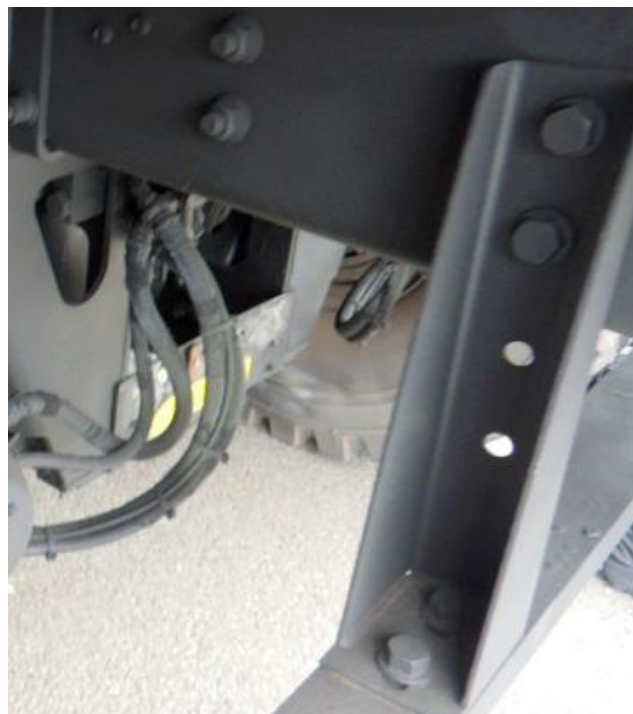
Figure 12. MTVR Under-Ride Bar Mounting Showing Four Mounting Fasteners Per Side Plus Two Additional Holes for Non-functional Fastener Sets (12 Total) Per Vehicle
