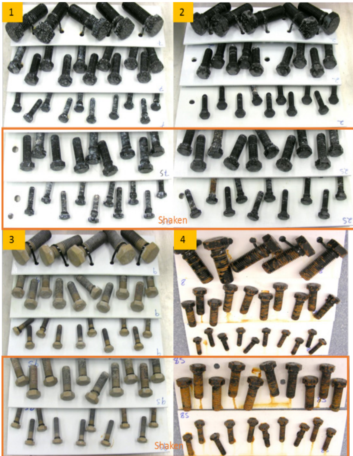
Figure 20. Cyclic Corrosion on Bolts (120 Cycles for All Except 40 for Set 4)
