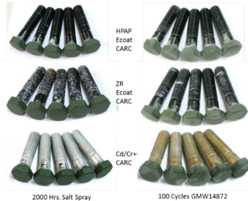
Figure 5. Corrosion Performance of Cadmium Plated, Hexavalent Chrome Rinsed Fasteners (Bottom), Inorganic Zinc Rich Primer with Electrodeposition Topcoat (Middle) and High Purity Aluminum Plating with Electrodeposition Primer (Top) After 2000 Hours Salt Spray (Left) or 100 Cycles GMW14872 (Right).
