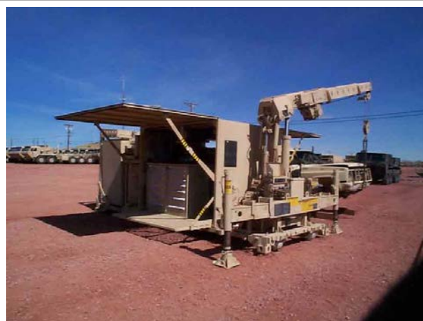
Figure 3. US Army Forward Repair System, manufactured by Rock Island Arsenal.
