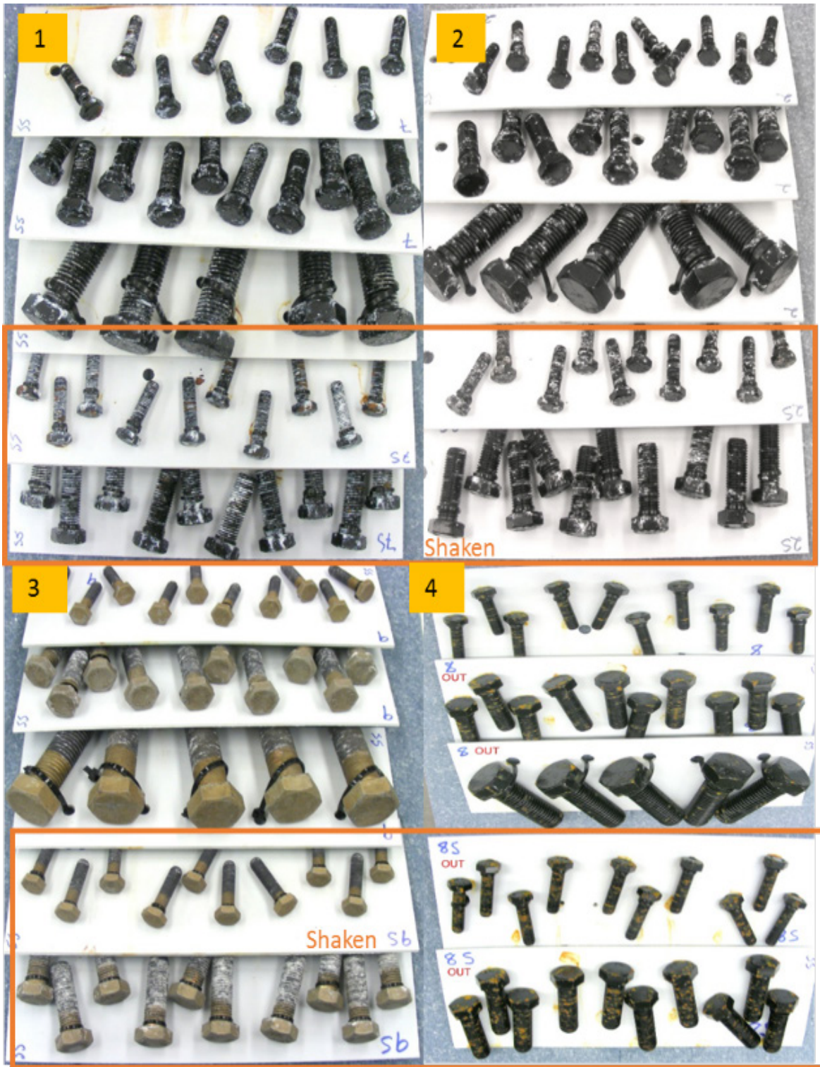
Figure 19. Salt Spray on Bolts (2000 hrs. for All, Except 500 for Set 4)
