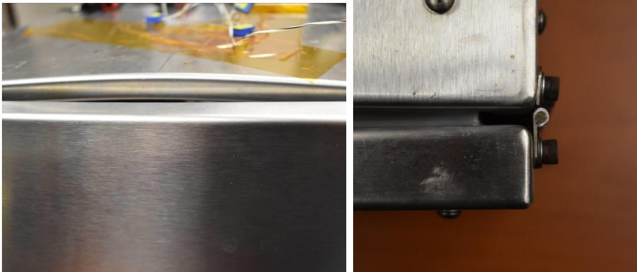
Figure 9 Chamber after testing with bulged top surface (left) and stretched hinge (right)
