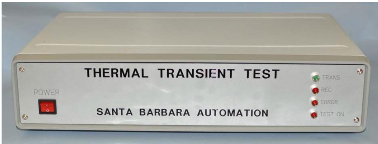
Figure 1 TTT system control unit
