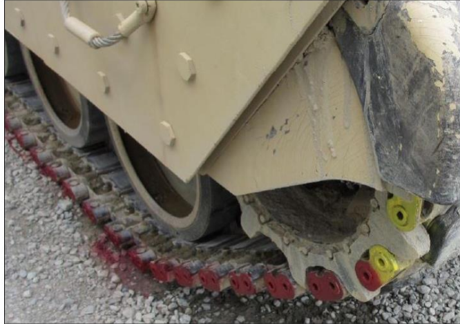
Figure 2. Prototype Track Pads in Bradley vehicle.
