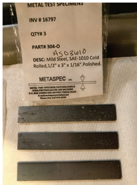
Figure 5. Post-test condition of 304-O test specimens.
