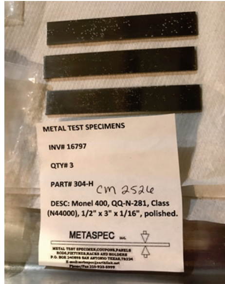
Figure 4. Post-test condition of 304-H test specimens.
