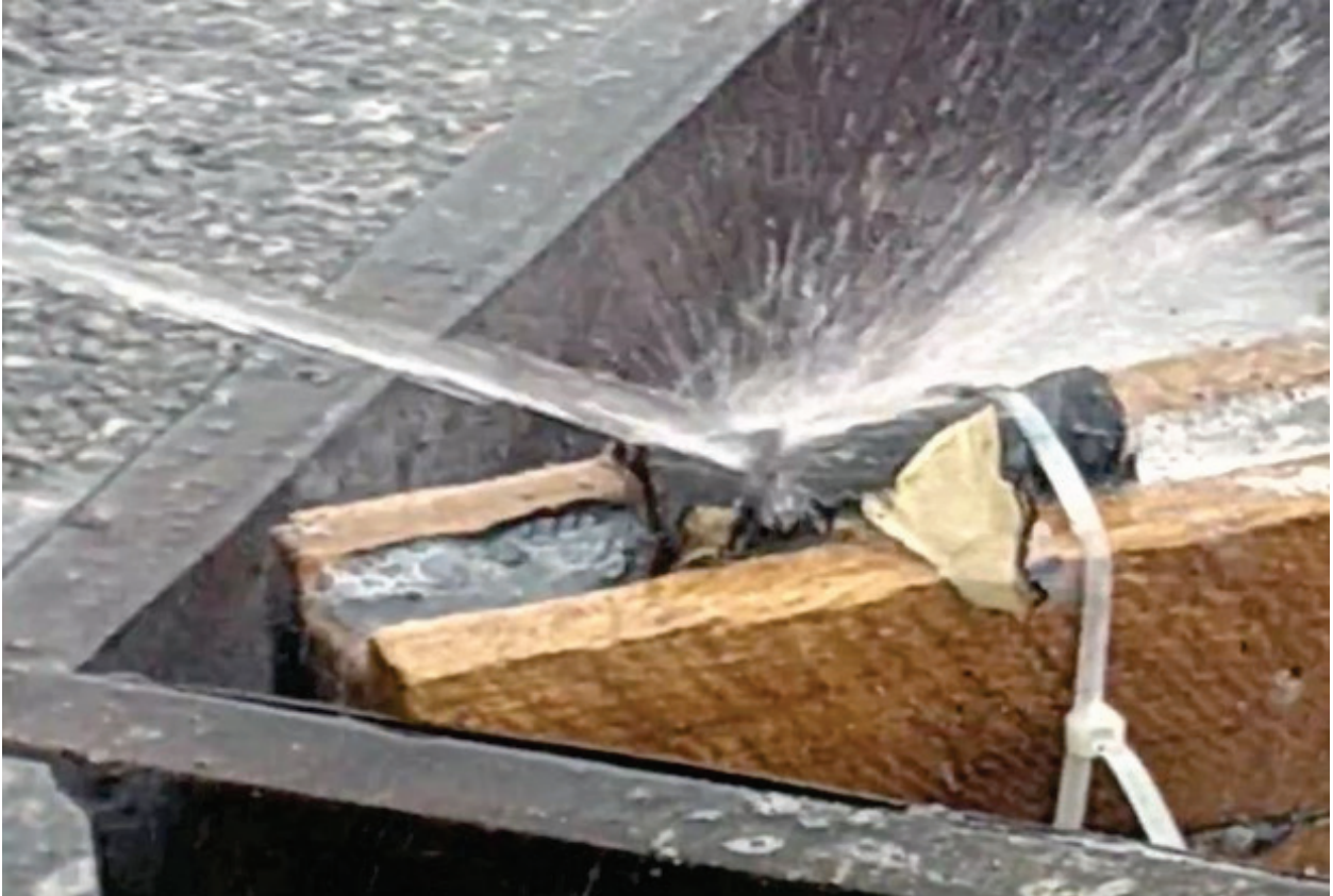
Figure 14. Thirty seconds after water application to ignited pyrotechnic underwater flare. Flare appeared to burn out after 30 s without any assistance from the water application.
