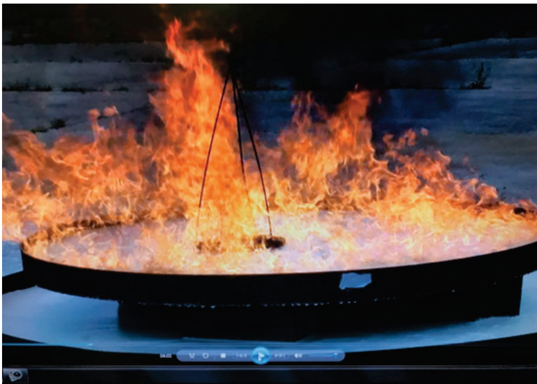
Figure 21. Burnback reignition of the fuel.
