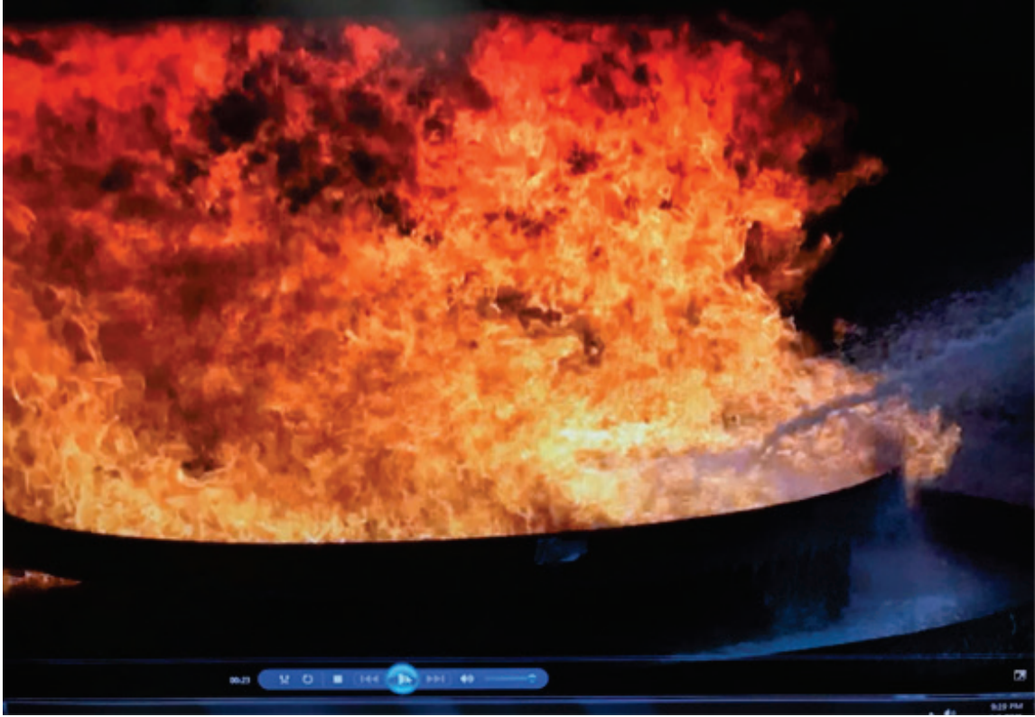
Figure 19. Full ignition of the fuel and initiation of first extinguishment.
