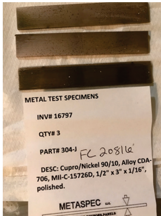
Figure 7. Post-test condition of 304-J test specimens.
