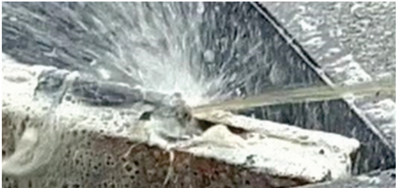
Figure 17. Three seconds after application of 10% BlazeCheck in water. Complete extinguishment without possible relight.
