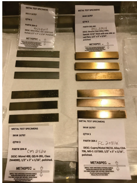
Figure 3. Post-test condition of the four test specimens.
