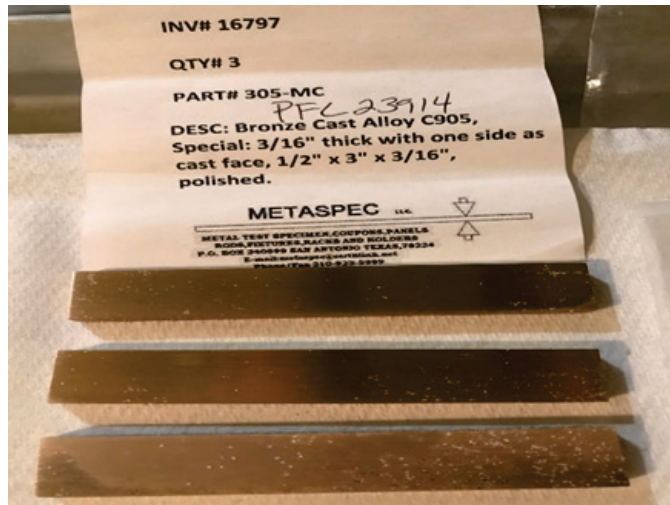
Figure 6. Post-test condition of 305-MC test specimens.
