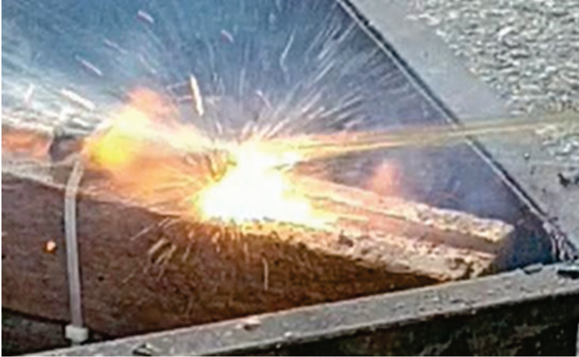
Figure 16. Time 0, start of application of 10% BlazeCheck in water.
