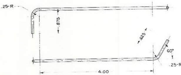
② WIRE (FOR BAND 1 - UPPER) #12 (.080) COPPER WIRE TINNED 1 REQ'D
