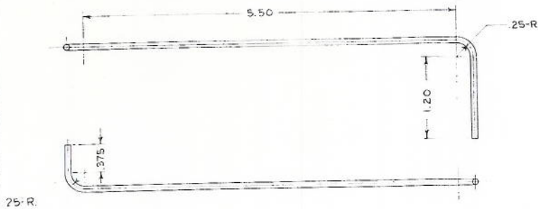
⑧ WIRE (FOR BAND 4 - RIGHT) #12 (.080) COPPER WIRE TINNED 1 REQ'D
