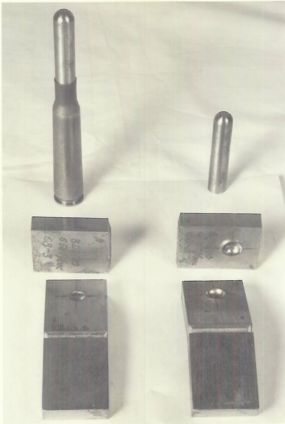
SPECIMENS AND PROJECTILES FOR BALLISTIC BEND TESTS ON STEELS.
