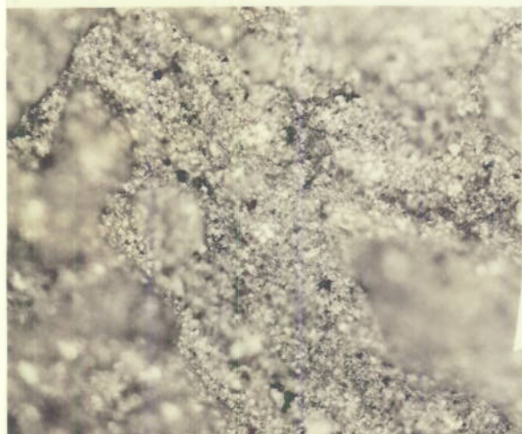
FRACTURES OF TEMPERED MARTENSITE IN A TEMPER BRITTLE CONDITION PLATE 52151, TREATMENT E. MAGNIFICATION 50.
