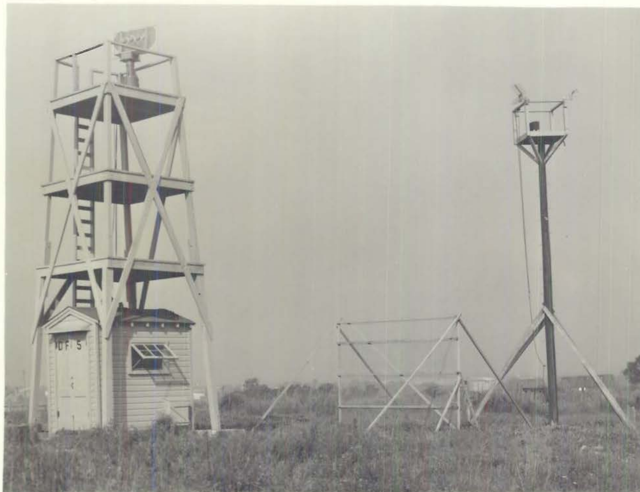
FIELD TEST INSTALLATION EXTERIOR VIEW SHOWING ROTATING MOUNT, SCREEN AND TRANSMITTING ANTENNAS
