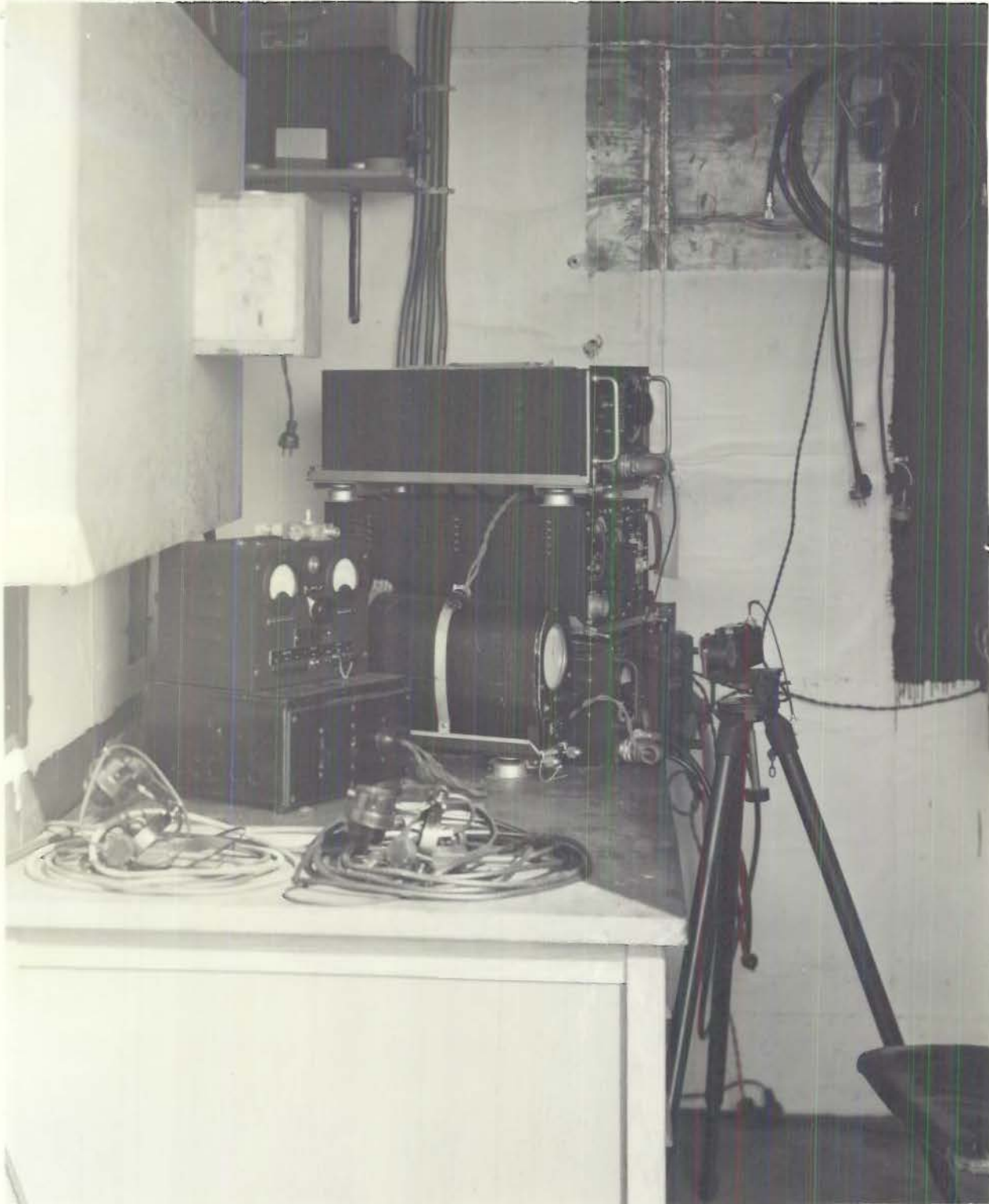
FIELD TEST INSTALLATION INTERIOR VIEW SHOWING RECEIVERS, INDICATOR MOTOR CONTROL DEVICE AND CAMERA.
