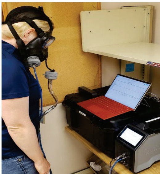
Figure 1: Demonstrating the use of the OHD QuantiFit2 fit test system for a gas mask
