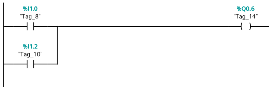
Figure 21. Simple OR Boolean Logic Operation in a LAD Network
