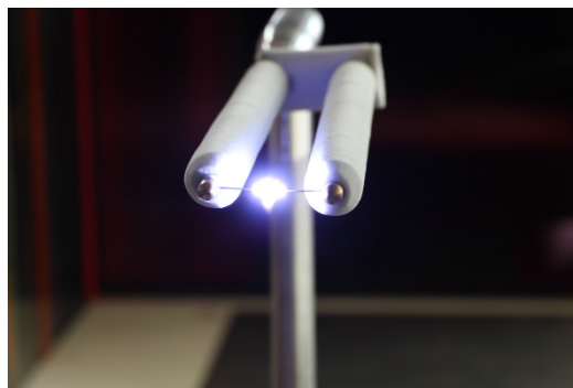
Figure 2-22: New SPARC Source Especially Designed for AVT233 Tests.
