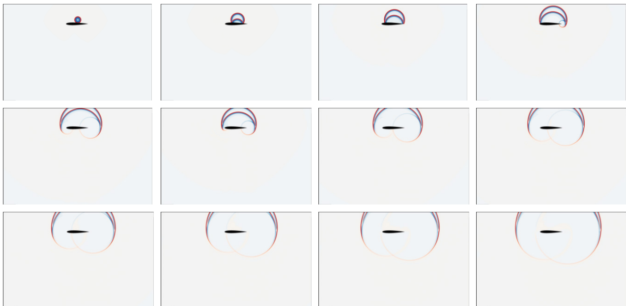
Figure 3-33: Numerical Simulation of Propagation of Pressure Signal Induced by Laser Pulse Source, DLR CAA Code PIANO.
