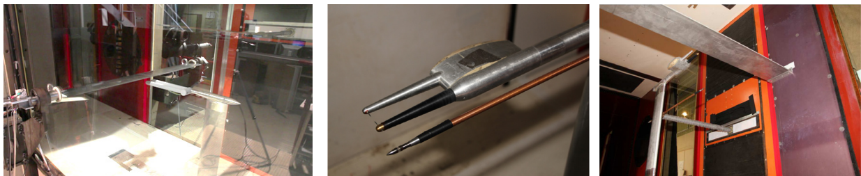
Figure 2-18: SPARC Source in F2 for Preliminary Tests with Plane Plate.
