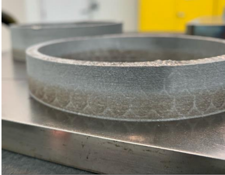
Fig. 4 Premature print failure due to uneven powder dispersion caused by a heavily worn elastomeric recoater
