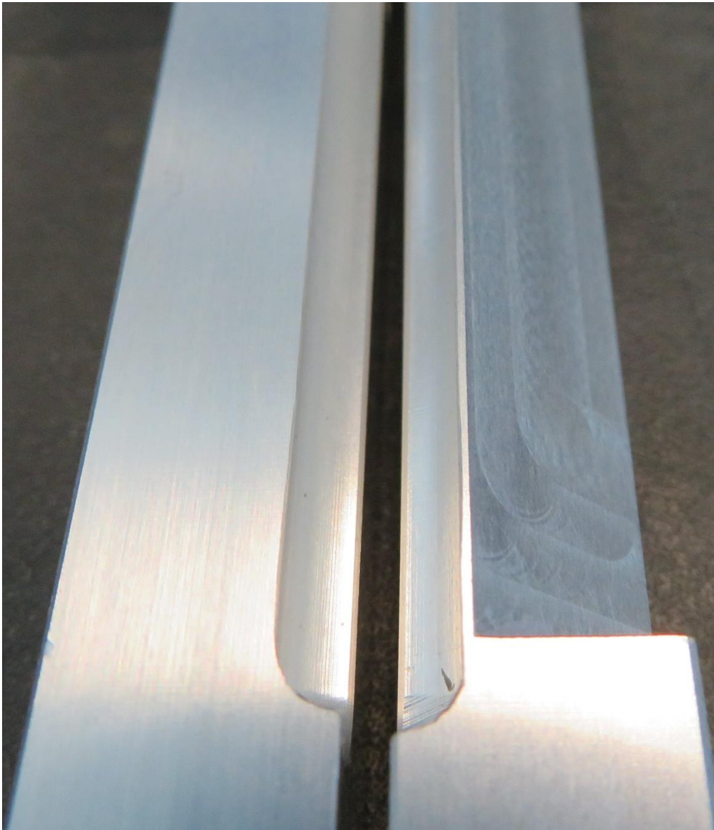
Fig. 1 Aluminum recoater arms with grooves
