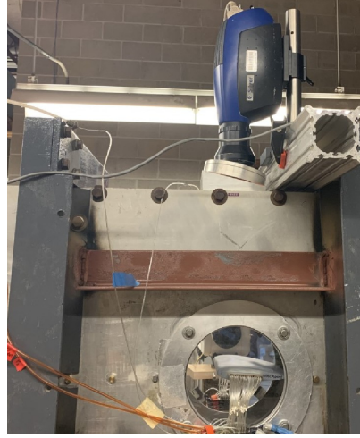
Figure 2.6: Setup of the infrared camera for airfoil surface temperature measurements during the wind tunnel experiment.
