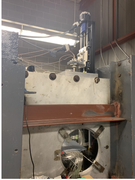
Figure 2.9: Traversing wake rake installed in the test section for wind tunnel experiments.
