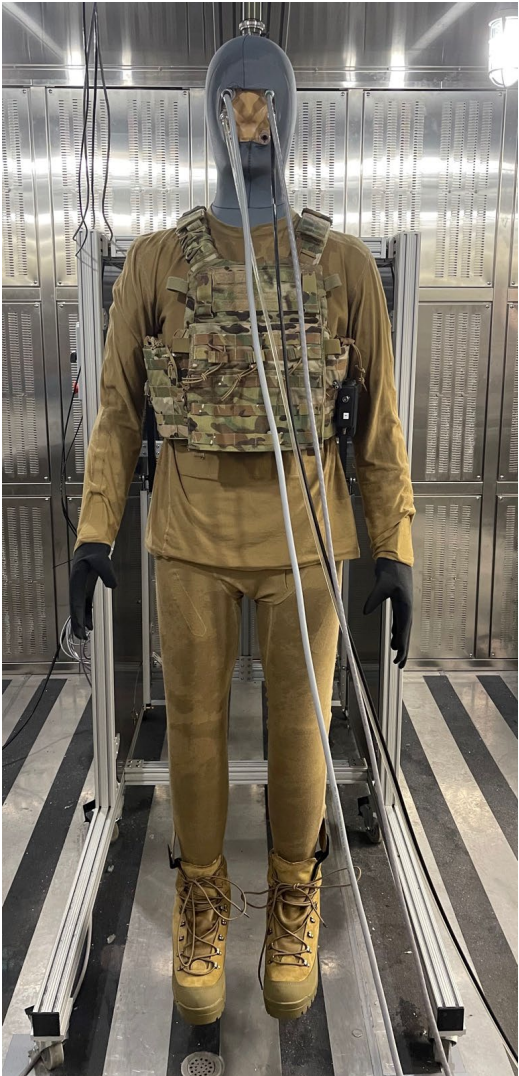
Unpowered Heated Base Layer Ensemble (TacHEAT, Human Systems Engineering, Inc., Waltham, MA). This base layer ensemble is placed over the thermal manikin's sweating skin (see gray textile covering manikin head)
