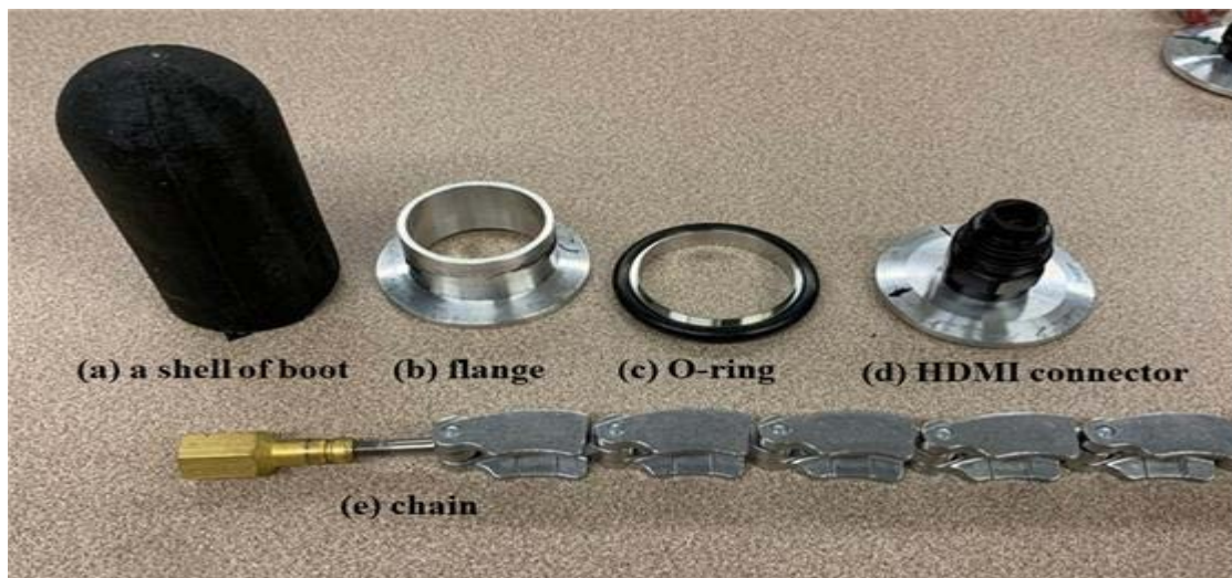
Figure 8. Components used for assembling sensor housing
