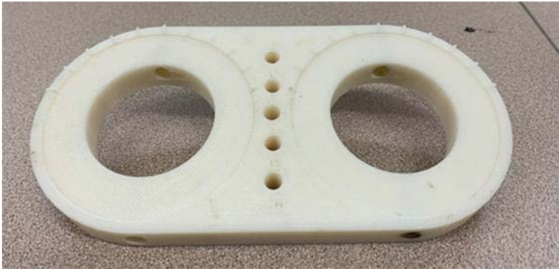
Figure 14. The 3D printed fixture for mounting the sensors.
