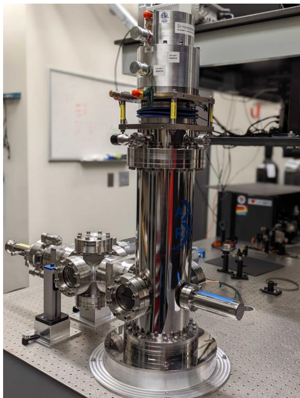
Figure 2. ARS cryostat on optical table in Bassett lab. The vertical tower is part of the UHV chamber, in which a cold plate is couple to the cold head using He exchange gas. The load lock extends to the left from the UHV chamber, and the glass optical cell (not pictured) will be attached in the place of the steel blank shown extending to the right from the UHV chamber.
