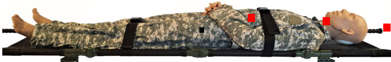
Figure 5. ISMv1.2 manikin, and sensor locations.
