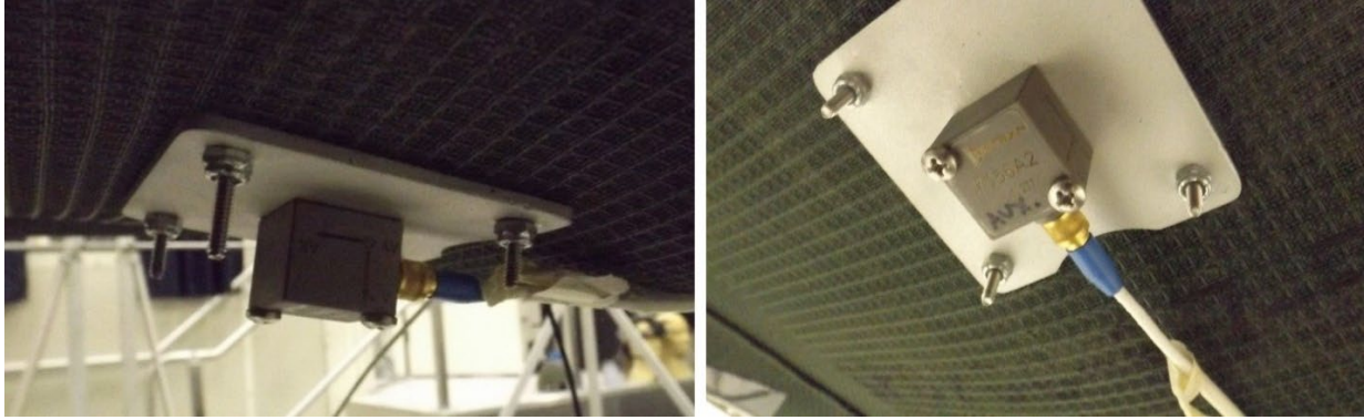
Figure 3: Location of the auxiliary sensor, and how it was mounted. This sensor was placed on the bottom of the litter mesh, and provided the measurements of the input vibration. As seen on the left, the wire was taped to the mesh to prevent wire motion from interfering with the sensor readings.
