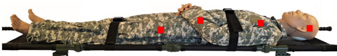
Figure 2: Instrumented Supine Manikin for Vibration (ISMV) in the two-strap condition with the body segment sensors identified by red squares. From left to right, the identified segments are the thigh, pelvis, chest, and head. The sensors are internally located for the ISMV, and externally located for the human subjects.
