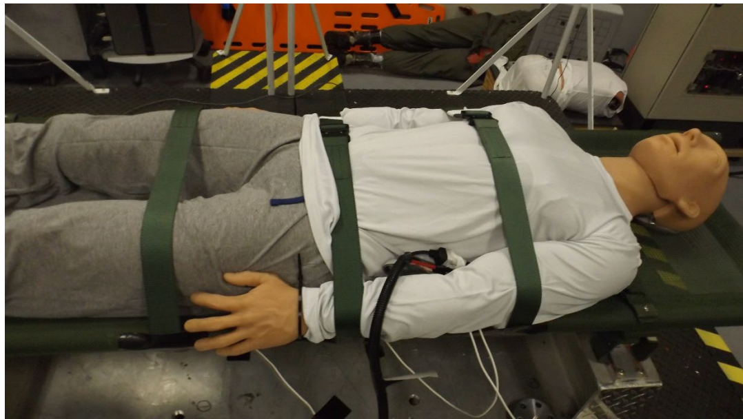
Figure 8. Day 2 litter strap securing method for Phase 2.
