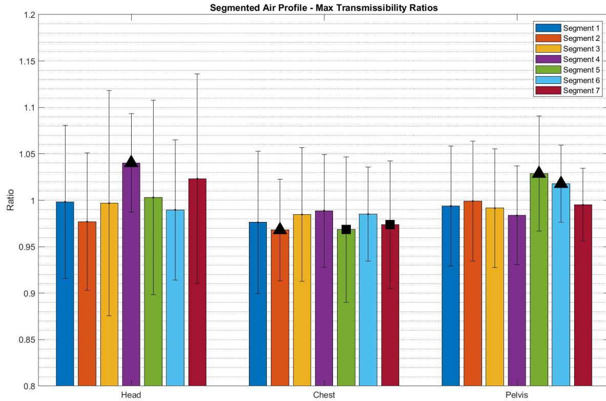
Figure 18: This figure depicts the mean ratio values and corresponding standard deviations of the max transmissibility ratios for the head, chest, and pelvis body segments over the seven time segments of the Air vibration profile. The bar shows the mean ratio, the black brackets show the corresponding standard deviation, the black triangles denotes statistically significant results, and the black squares denote results of marginal statistical significance.
