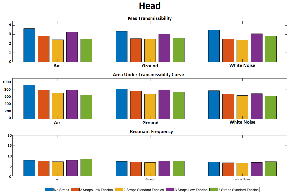
Figure 18. Bar plots comparing metrics calculated from the manikin's head transmissibility plots.
