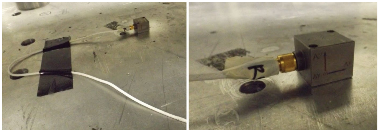
Figure 4: Location of the vibration table sensor, and how it was mounted. The wire was taped to the table to prevent wire motion from interfering with the sensor readings.
