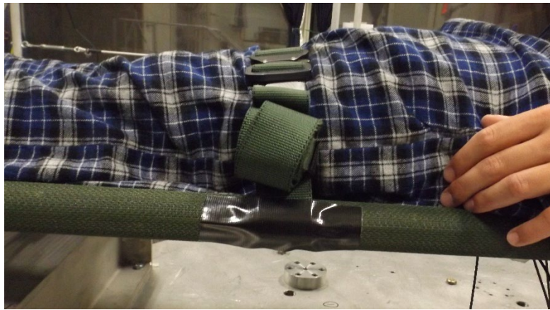
Figure 15. Tape to secure litter strap to litter for Phase 3.
