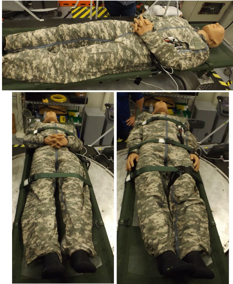
Figure 1: Images of the three utilized strap conditions. At top is the no strap condition, left is the two-strap condition, and right is the three-strap condition.
