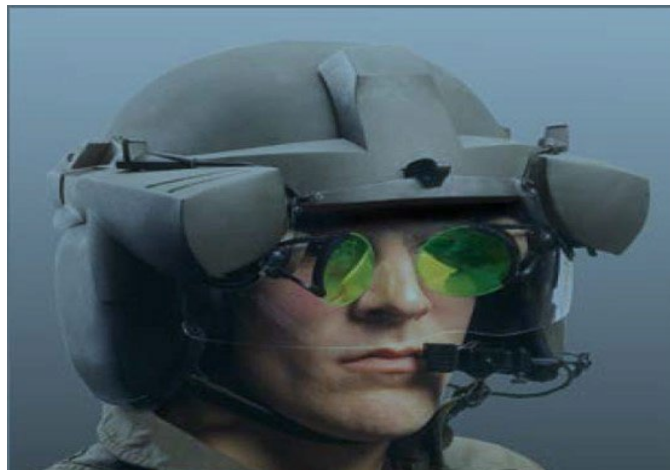
Figure 1. RAH-66 Comanche HIDSS prototype consisting of two monoculars with overlapping FOV.
