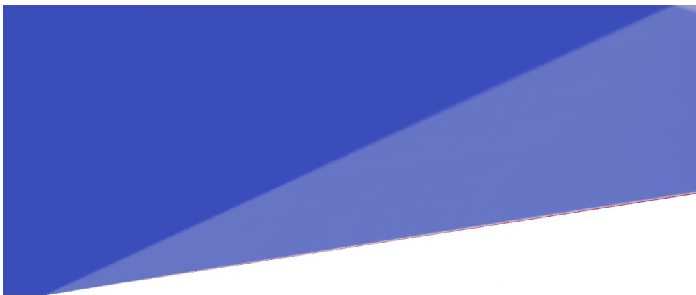
Fig. 25—Temperature profile for a 10^\circ oblique wedge moving through quiescent air at 3 km altitude at M = 3 . The temperature range is 268 K (blue) to 750 K (red, at the wedge surface).
