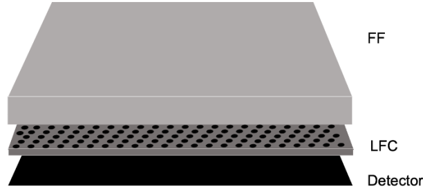
Figure 2: Experimental design for the physical CNR measurements using the LFC phantom. SNR measurements were performed without the LFC in place.
