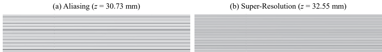
Figure 6. VCT simulations of a 7.0 \text{ mm}^{-1} bar pattern phantom illustrate the z -dependency of super-resolution in the reconstruction.
