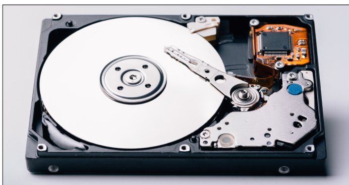
Mechanical hard disk computer drive – uses rare earth element magnets.
