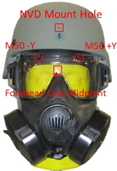
Figure 113. ACH medium with M-50 JSGPM mask with red squares that identify the M-50 JSGPM mask +Y and –Y points, the ACH NVD mount hole point, and the forehead midpoint locations. The length between the forehead midpoint and each of the three helmet points was calculated for each helmet mount pre- and post-mass properties measurements.
