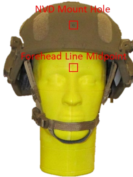
Figure 57. IHPS with the red squares identifying the NVD mount hole and forehead midpoint location. The length between the two points was calculated for each helmet mount pre- and post-mass properties measurements.
