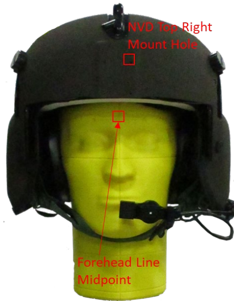
Figure 101. HGU-56/P aviator helmet with red squares that identify the helmet +Y and –Y points, the NVD top right mount hole point, and the forehead midpoint locations. The length between the forehead midpoint and each of the three helmet points was calculated for each helmet mount pre- and post-mass properties measurements.
