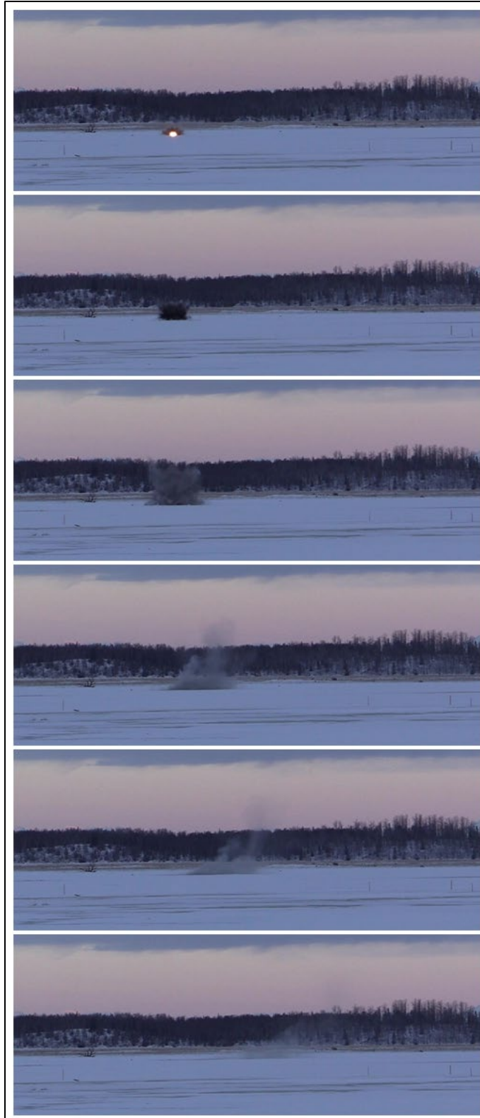
Figure B-6. Progression ( top to bottom ) of a postdetonation cloud immediately following impact of an 81 mm IMX-104 cartridge from this study.
