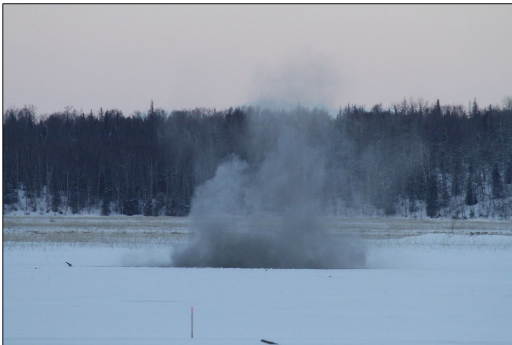
Figure B-3. Example 3 of a postdetonation cloud immediately following impact of an 81 mm IMX-104 cartridge from this study.
