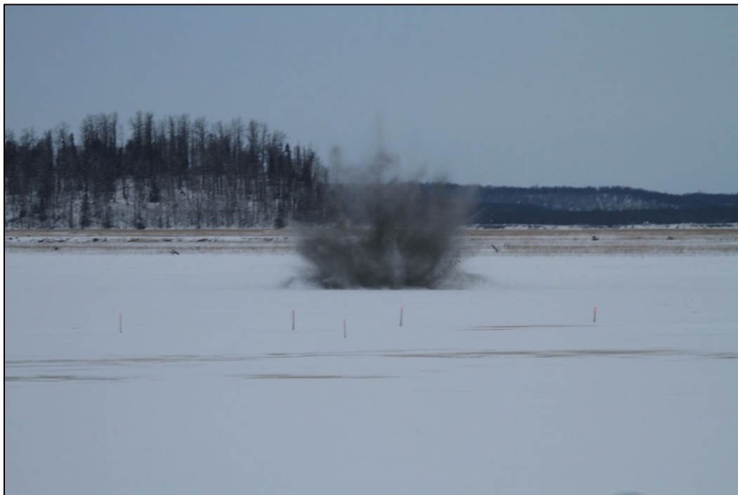
Figure B-1. Example 1 of a postdetonation cloud immediately following impact of an 81 mm IMX-104 cartridge from this study.
