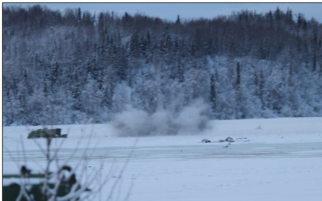
Figure B-4. Example 4 of a postdetonation cloud immediately following impact of an 81 mm IMX-104 cartridge from this study.
