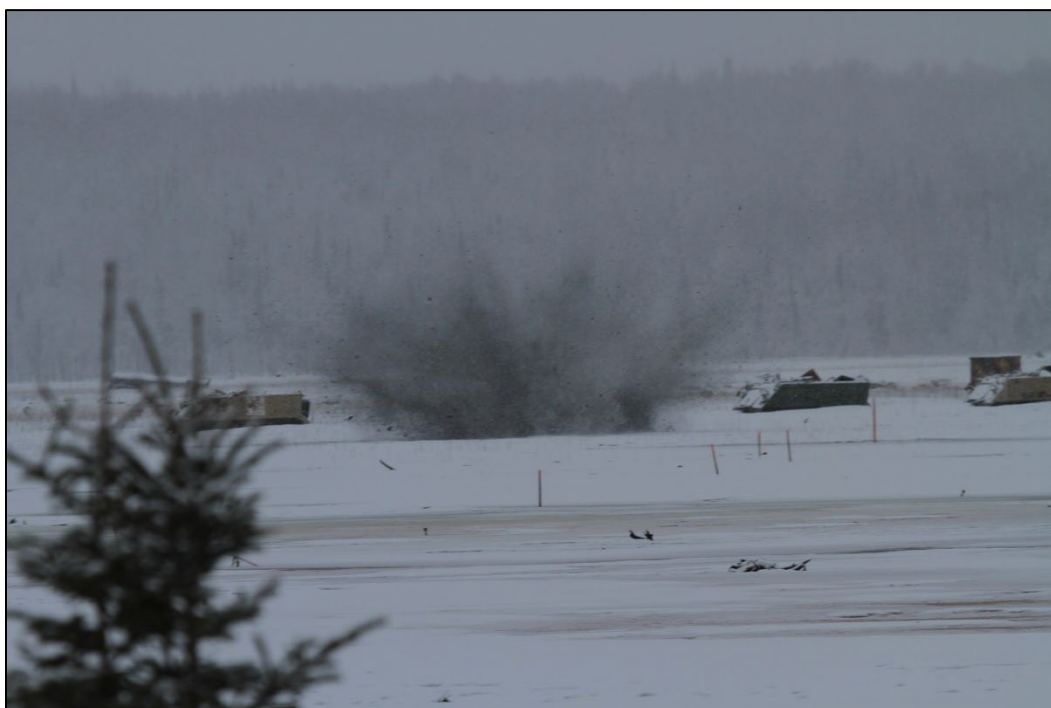
Figure B-2. Example 2 of a postdetonation cloud immediately following impact of an 81 mm IMX-104 cartridge from this study.
