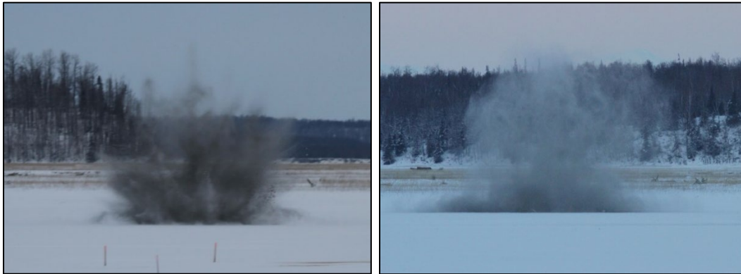
Figure 3. Two examples of postdetonation residue, soot, and gas clouds from live fire of 81 mm IMX-104 (M889A4) cartridges.
