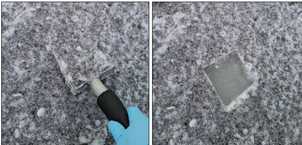
Figure 5. An example sample increment from Plume 10, showing the thin snow layer and subsurface ice typical of Plumes 6–13.
