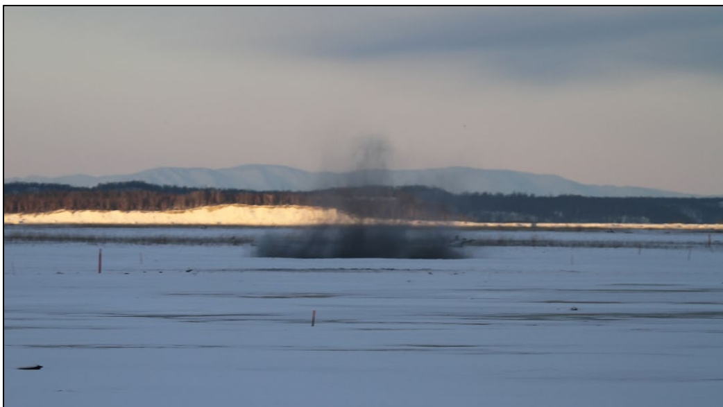
Figure B-5. Example 5 of a postdetonation cloud immediately following impact of an 81 mm IMX-104 cartridge from this study.
