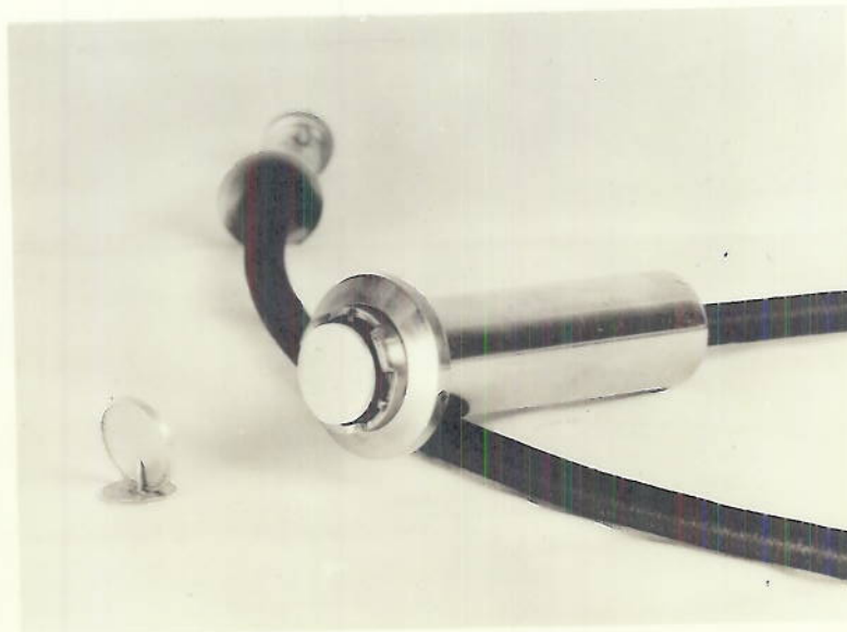
FIG. 2 DURALUMIN FILLER - ATTACHED TO PROBE
