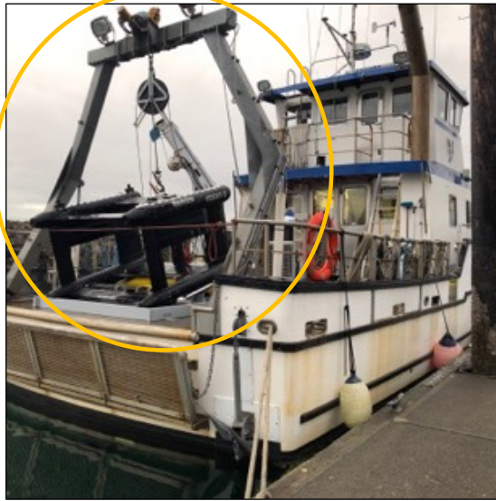
Multi-Sensor Towbody (MuST), developed by the Applied Physics Laboratory, University of Washington
