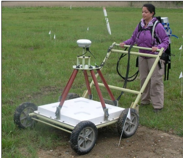
Time-domain Electromagnetic Multi-sensor Towed Array Detection System (TENTADS), developed by the Naval Research Laboratory and Nova Research
