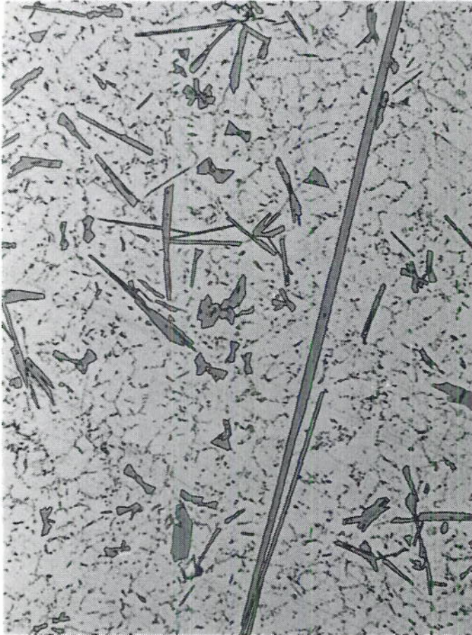
FIG. 1 PRIMARY CRYSTALS OF Fe_2Al_7 IN EUTECTIC Al-Fe_2Al_7 . CAST IN PERMANENT MOLD - Fe 5%, Si 0.04%, 250 X, 0.5% HF ETCH.
