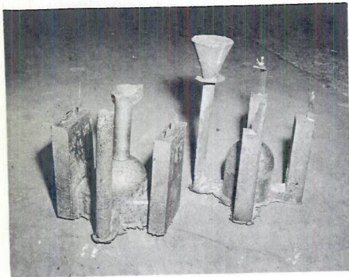
TYPICAL CASTINGS USED TO PROVIDE MATERIAL FOR STRESSED GRAPHITIZATION TEST FIXTURES.
