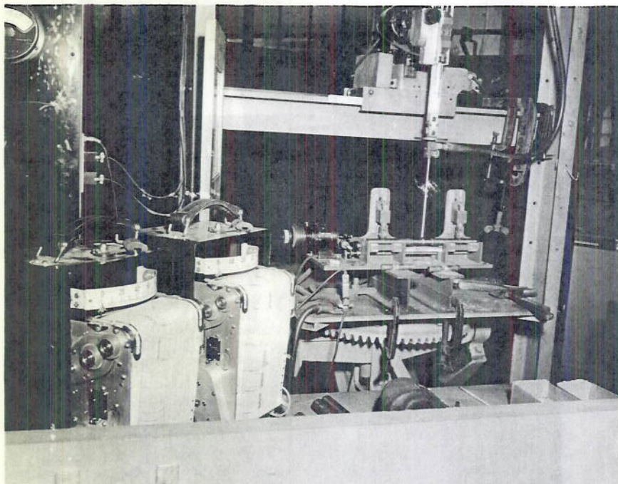
VIEW OF AUTOMATIC WELDING MACHINE AND INSTRUMENTS FOR MEASURING AND RECORDING THE CURRENT AND VOLTAGE.
