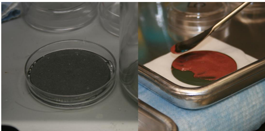
Figure 5. DD on the surface of an SS coupon (left), and SDS decontaminant being applied to the surface of a PU paint-coated coupon (right).
