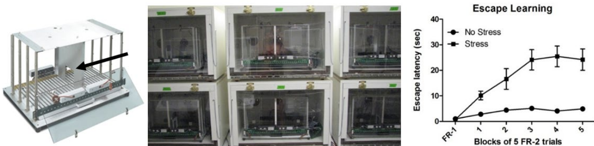
Figure 3. Left – The shuttle box has two chambers with a small opening between them and an electrified grid floor. Right – Performance in the standard Shuttle Box Escape task is shown to degrade when the subject is exposed to a stressor.
