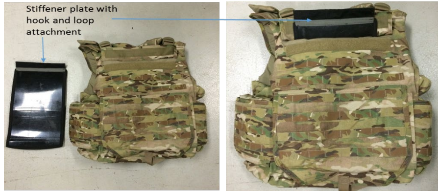
Figure 3. The IOTV pictured with plastic plate used to provide additional stiffness to the back pocket where the DWD sheath was attached.
