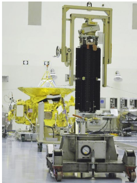
Figure 6. New Horizons and its GPHS RTG. Source: [13].
