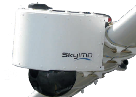
Figure 37. TASE 200 sensor in SkyIMD enclosure
