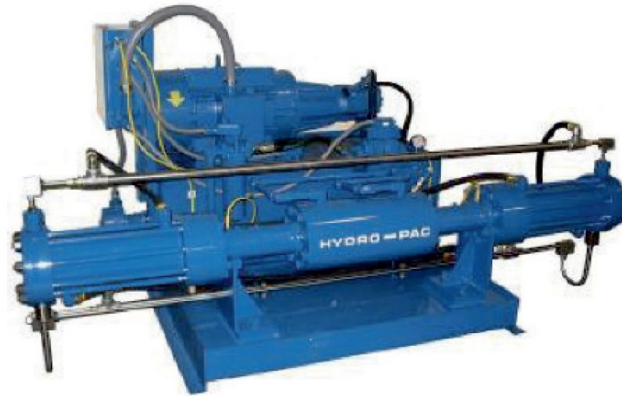
Figure 14. Hydrogen Gas Compressor. Source: Hydropac (2010).
