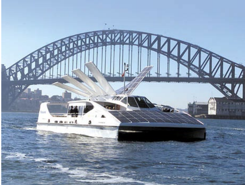
Figure 2. Passenger Ferry Equipped with Photovoltaic Solar Panels. Source: Solar Sailor (2015).
