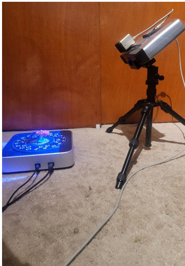
Figure 28. EinScan Pro used to reverse engineer commercial components.
