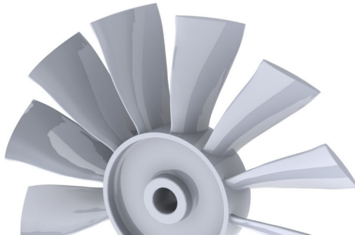
Figure 32. Final CAD model of the fan rotor.
