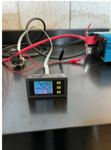
Figure 4.10. Bidirectional volt/amp meter
