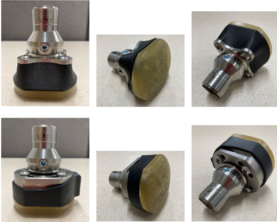
Figure 3: “Dummy” (top) and Instrumented (bottom) prostheses for the sheep. The “dummy” prosthesis includes a 3D-printed metal plate for structure, a polyurethane tread molded over it, and a nylon 3D-printed spacer with pressed-in inserts for strength and to match weight. The Instrumented prosthesis uses the Europa+ Smart Pyramid and a matching polyurethane tread. The prosthesis adapter on top attaches to the osseointegrated prosthesis abutment.
