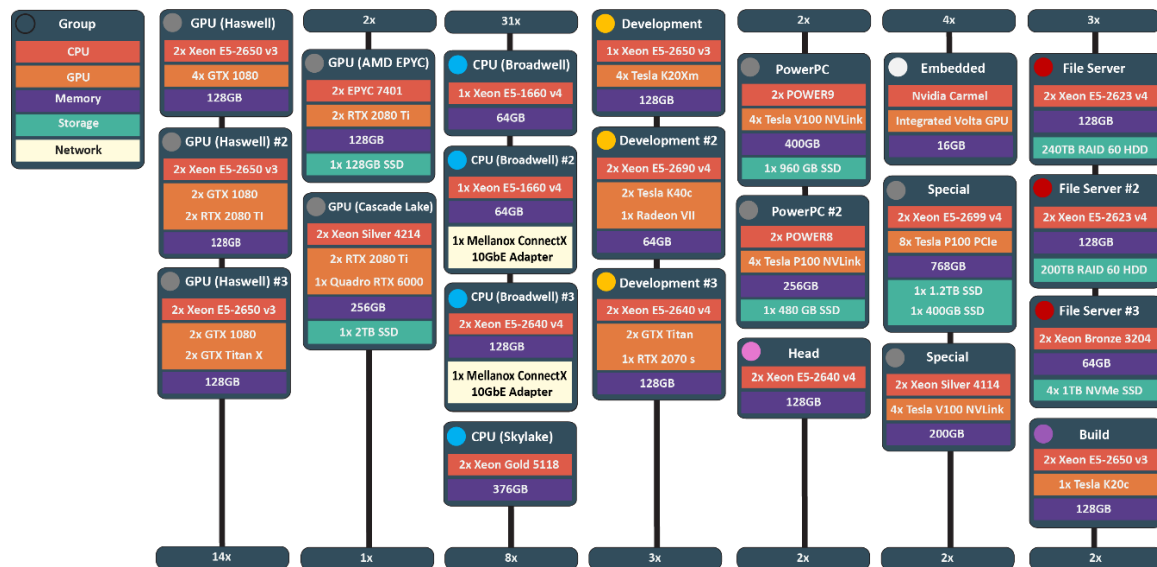
Figure A. Schematic of Euler. The CPU-GPU cluster has more than 80 GPU cards using the Maxwell, Pascal, Volta, and Ampere architectures.
