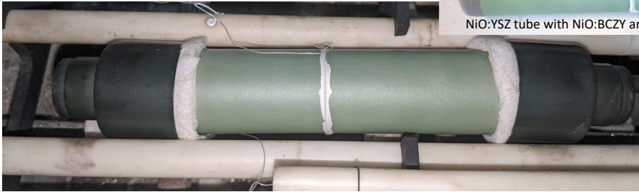
Figure 6 - Reduction of tube with proton conducting electrolyte versus standard YSZ electrolyte
