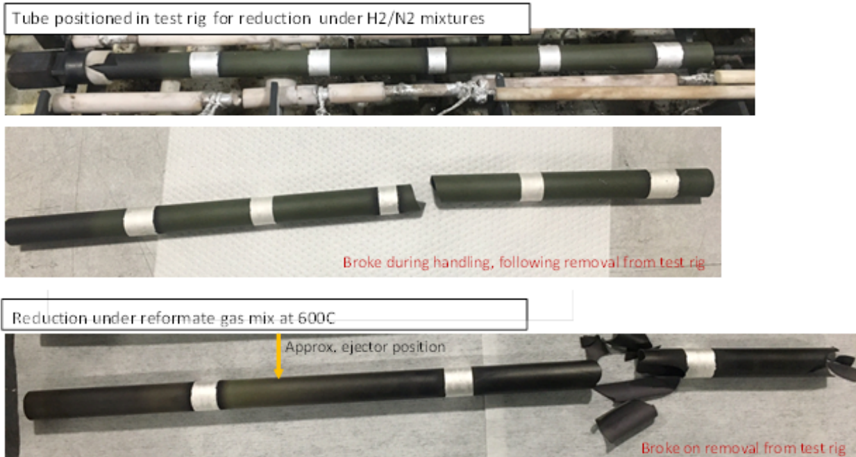
Figure 4 - BCZY:NiO tube with interconnect bands overcoated with silver ink reduced in test rig under H 2 /N 2 mixtures
