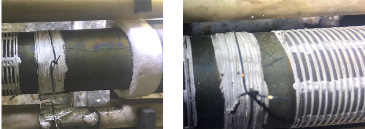
Figure 15 - Representative tube cracks following reduction and electrochemical testing.
