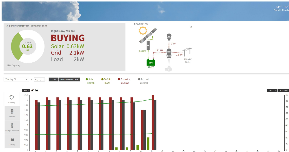
Figure 3.12. OpticsRE provides the user of this microgrid the ability to view and control certain functions from a remote location.
