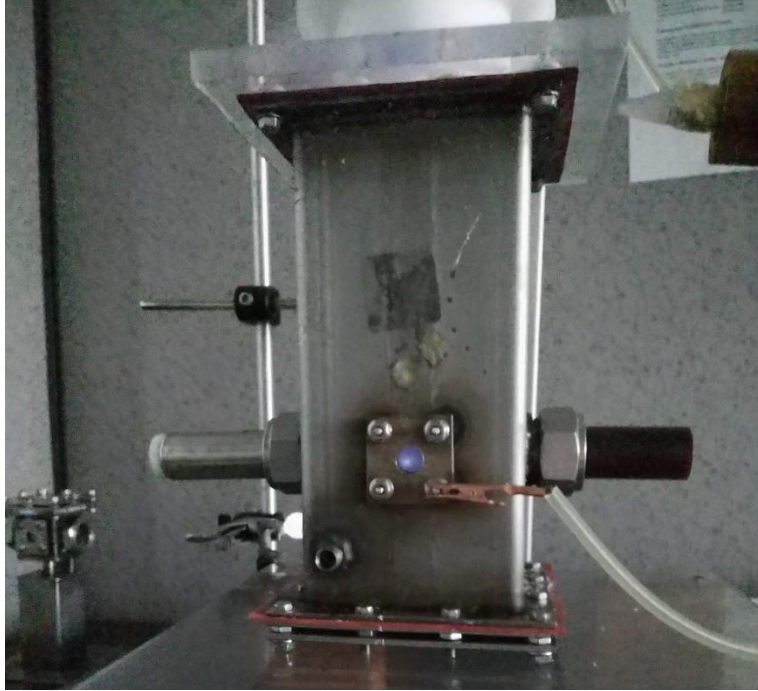
Figure 1. Schematic and photograph of an experimental setup for generation of corona discharge in liquid nitrogen
