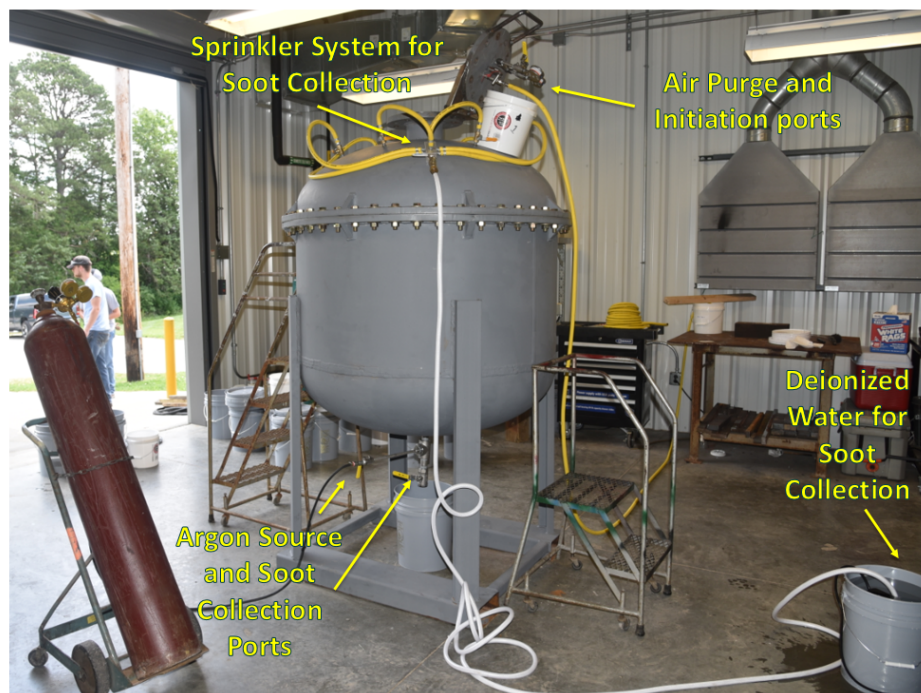
Figure 7. The assembled test chamber configuration after initial soot production tests
