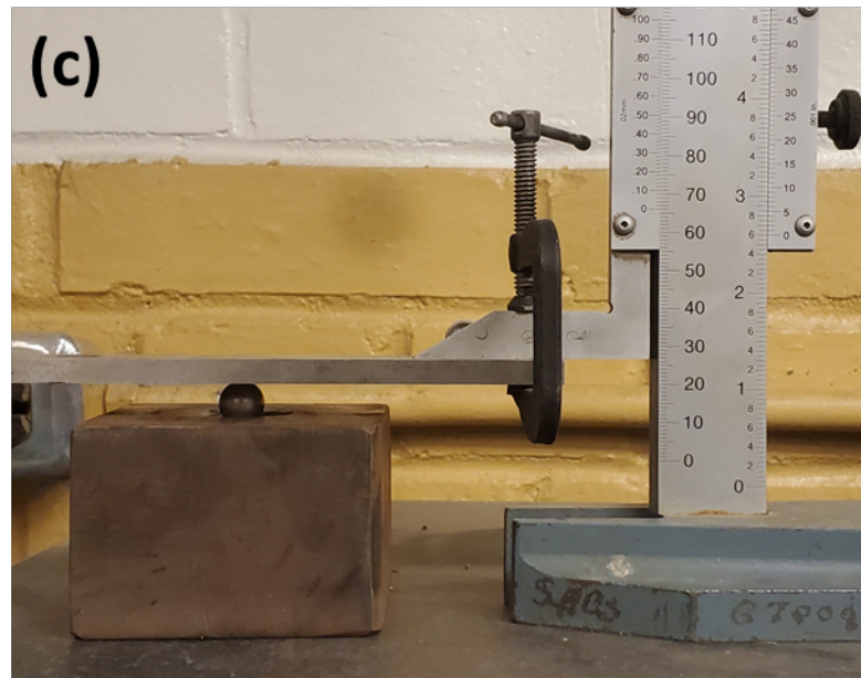
Figure 25. Cast 0.750 inch diameter x 1.000 inch long dent test pellet after removal from brass forming mold (a) and prepared dent test with piezoelectric pins attached for detonation velocimetry (b) and dent depth measurement using height gauge (c)
