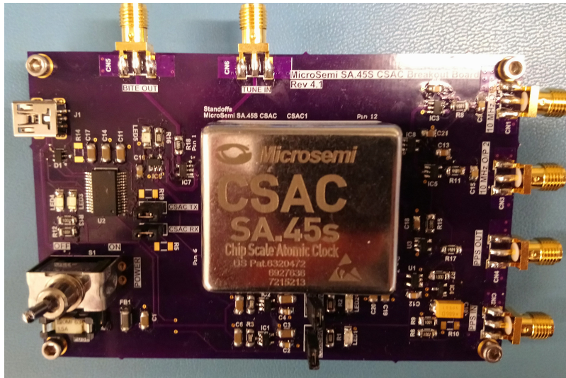
Figure 7. Assembled Interface Board
