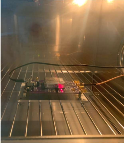
Figure 3. Image of CSAC inside of thermal chamber
