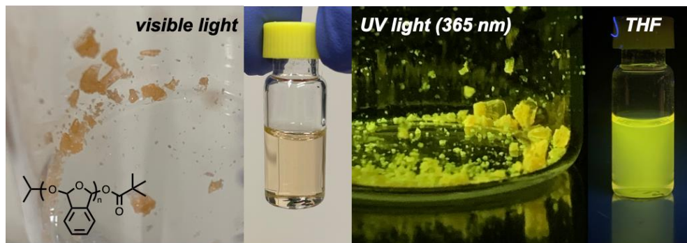
Figure 24. Images of IPA-PPA-Me 3 Ac as a glassy solid and in solution (3.5 mM in THF) under a UV lamp ( \lambda_{\text{exc}} = 365 \text{ nm} ).
