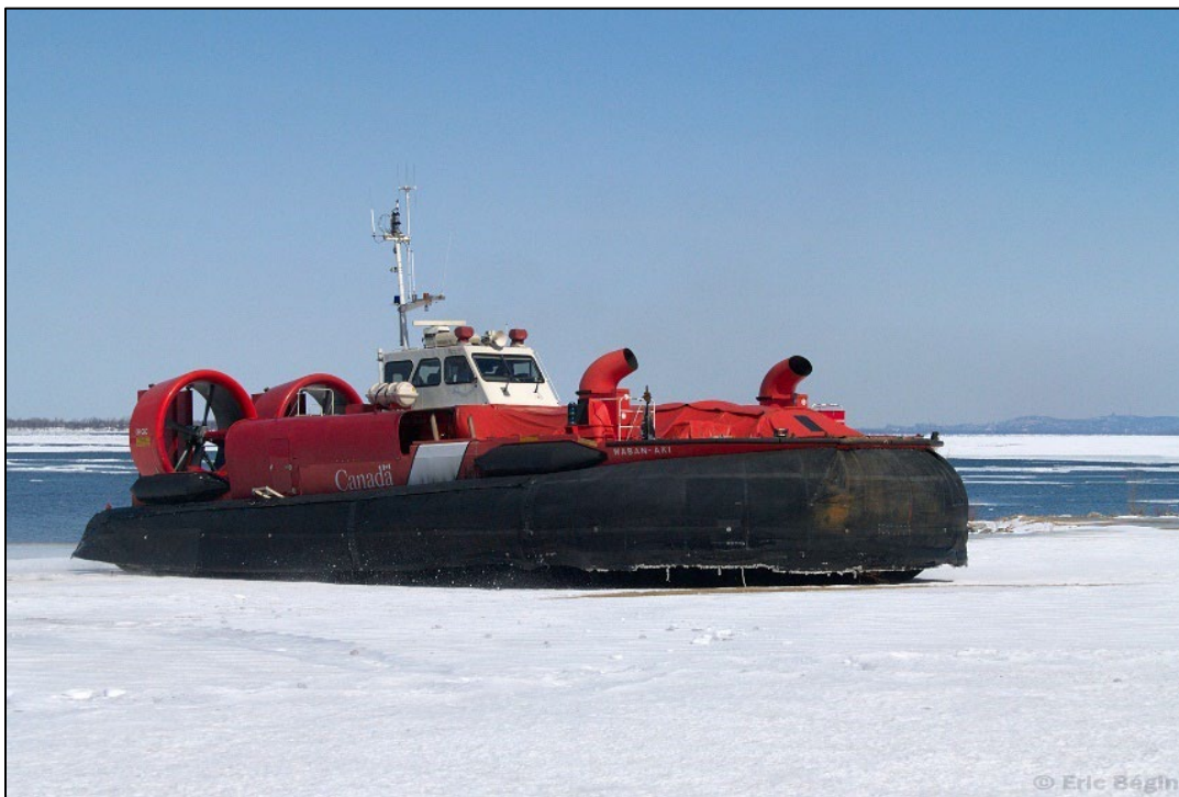
Figure 29. Hovercraft as an ice-breaking tool. (Image reproduced from Eric Bégin, Canadian Coast Guard WABAN-AKI , https://www.flickr.com/ Public domain.)
