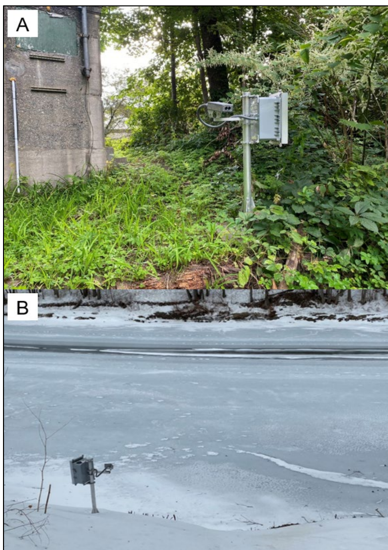
Figure 25. Example of single beam rangefinder (SBRF) installation position: SBRF instrument housing (A) and the SBRF placement next to the river with river ice present (B).
