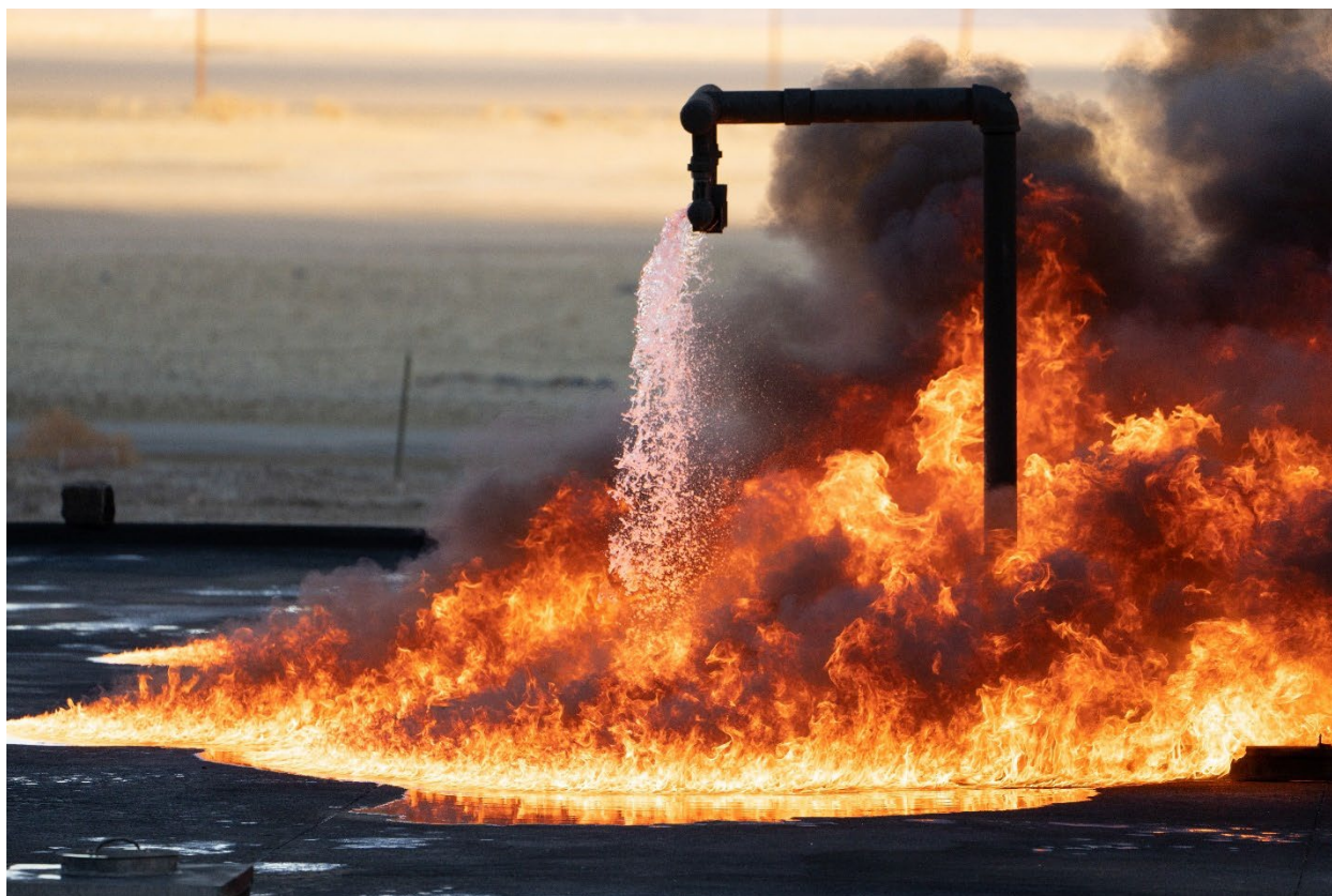
Fig. 4.6-1 – Flowing/Running Fuel Fire Scenario
