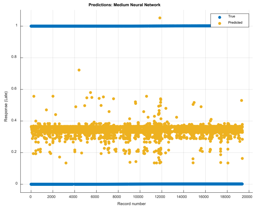
Figure 30. Graphical Representation of Medium Neural Network Model
