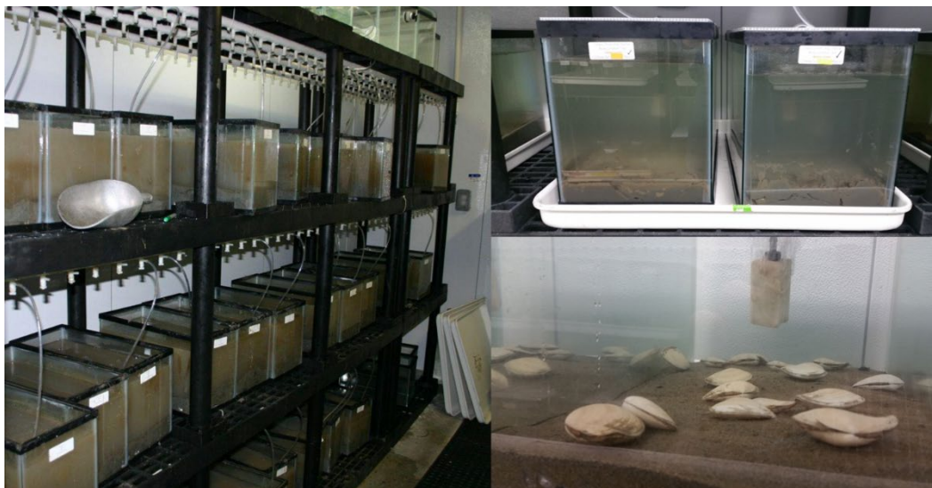
Figure 6-2. Laboratory whole-sediment bioaccumulation testing set up for a 28-day Macoma nasuta test. Note that the lower right image shows clams immediately following addition to the tanks; clams should be completely buried within 24 hours.
