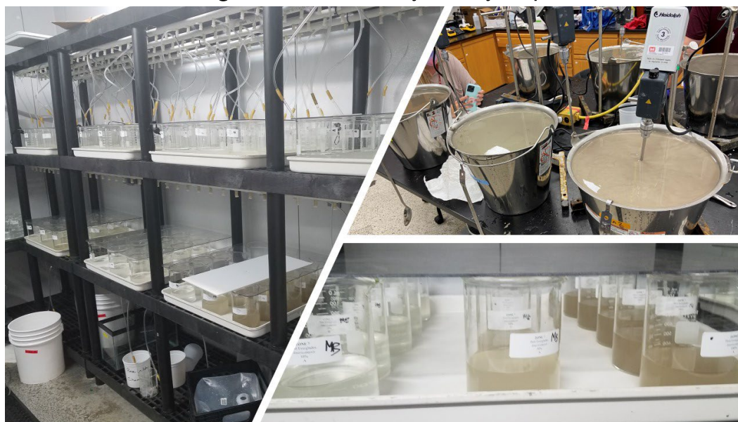
Figure 4-6. Elutriate toxicity bioassay setup.
