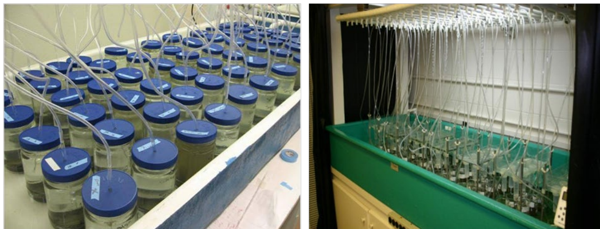
Figure 5-3. Laboratory whole-sediment sediment toxicity testing set up for a 10-day amphipod test ( left ) and a 10-day midge test ( right ) using a water-delivery apparatus.
