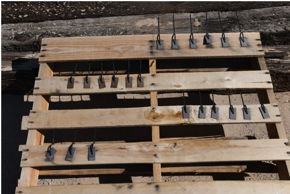
Figure 8. Outdoor test coupons at the site.
