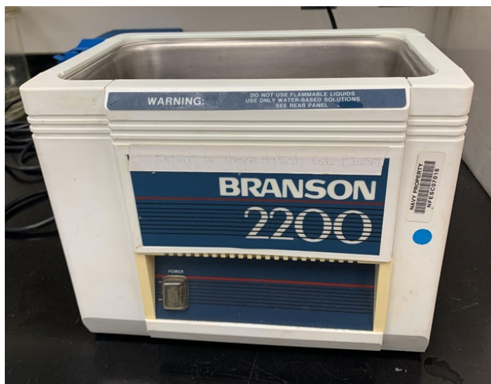
Figure 6. Branson 2200 ultrasonic cleaner.
